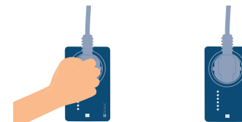
Figure 6 Plugging the device into the water protection switch
